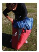
**Step 6.** Fold the wing with 3 or 4 folds whilst being careful to not crush the LE.
