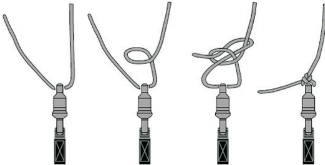
Figure: Bowline knot
