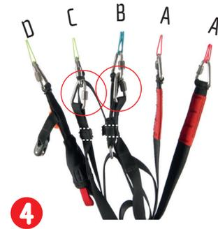
4 Attach bridle to the B & C riser carabiners and secure with the velcro straps
